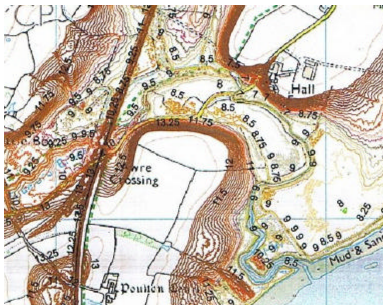
(Above) – satellite levelling plot for Gloucestershire WA land at Poulton Court prior to regulated tidal exchange
